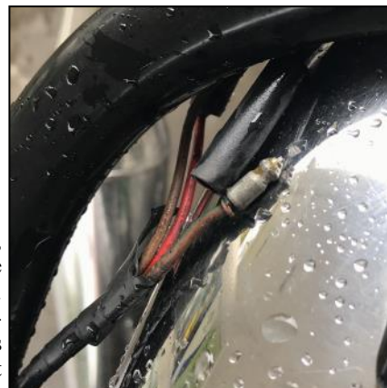
Right: Gremlin identified, and it really couldn't have been more out in the open. The old Lucas bullet terminal had come out of its connector at the tail light
