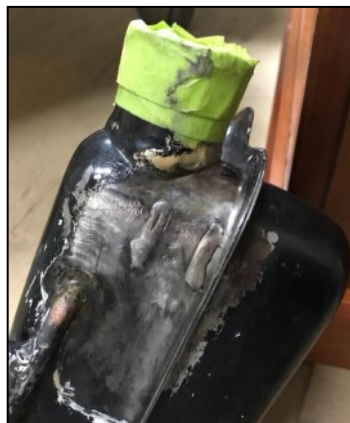
Left: The oil tank after removing the remains of the broken bracket and a bit of light wire wheel action.
