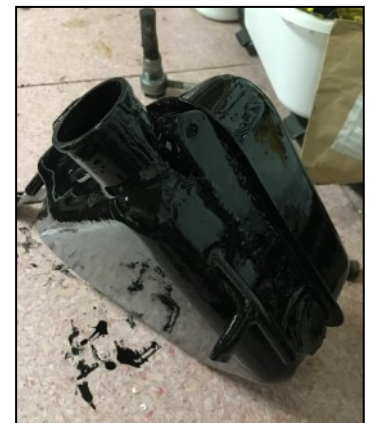
Left: The oil tank after removing the remains of the broken bracket and a bit of light wire wheel action.
