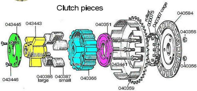
So, here's the culprit. The clutch spider (043443) had broached completely through and the full 60ft-lb was pressing clutch spider on the output shaft of the gearbox (shown in green in the previous diagram.
