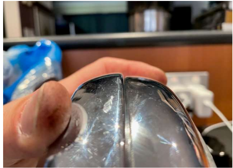
Old vs New Headlamp Rim - Just a poompteenth off, but enough so it won't fit.
