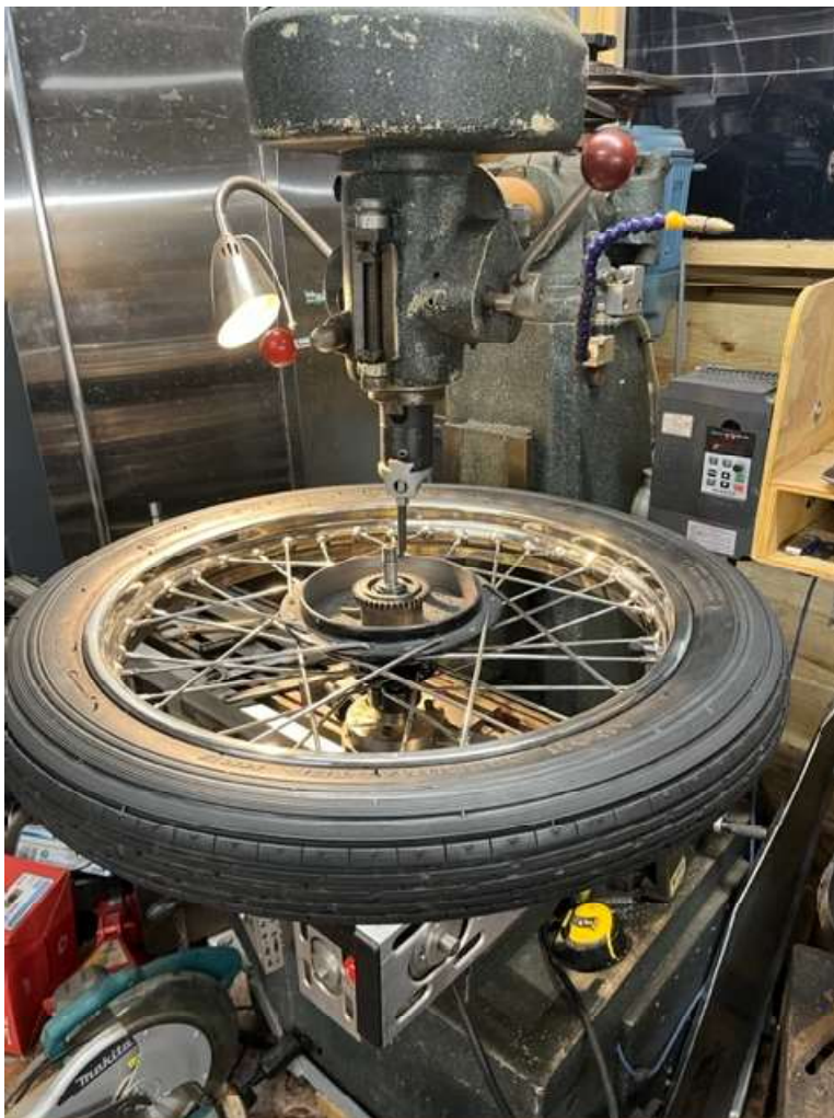
Cap over the bearing keeps the iron swarf out the bearing.
