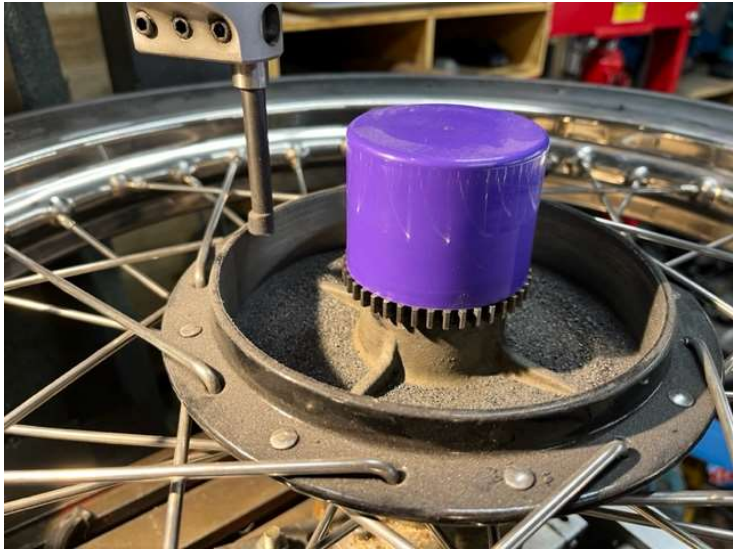
Cap over the bearing keeps the iron swarf out the bearing.
