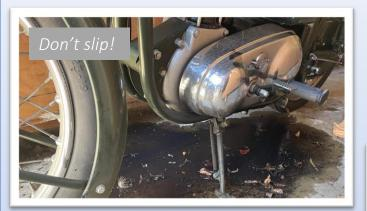
A quick search revealed the 'New British Motorcycle Anti-Wet Sump Valve Kit' (around AUD\$160), manufactured in England and made of aluminium. Apparently, the check ball valve will hold the oil in the oil tank where it belongs, then when started the pump suction will open the valve. This pump needs to be primed once after installation. Has anyone had any experience with these? I get a lot of conflicting information from the internet forums about their safety and efficacy...
