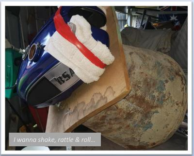
bolted down on the agitating paddles of the mixer bowl as it was a BSA tank it has one central mount point so a length of "all thread" from the board up into the tank and a failsafe strap over the top of the whole lot in case it broke free.
